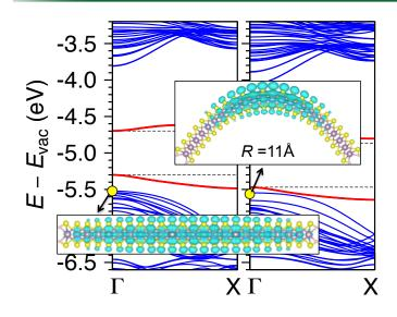
Bending induced charge localization and Fermienergy level shift in armchair 1H-MoS<sub>2</sub> nanoribbon. The lower red-curve corresponds to the occupied edge states whose energy decreases with increasing bending curvature. The wave functions of top non-edge valence bands get localized to the middle region of the nanoribbon when bending is applied.
